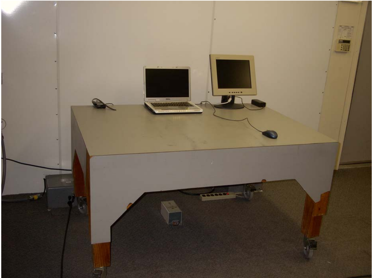
AC Conducted Emissions Measurement (Front View) Setup
