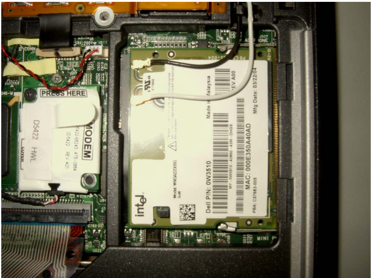
View of the WLAN Transmitter Location Inside the Laptop (Close-Up)
