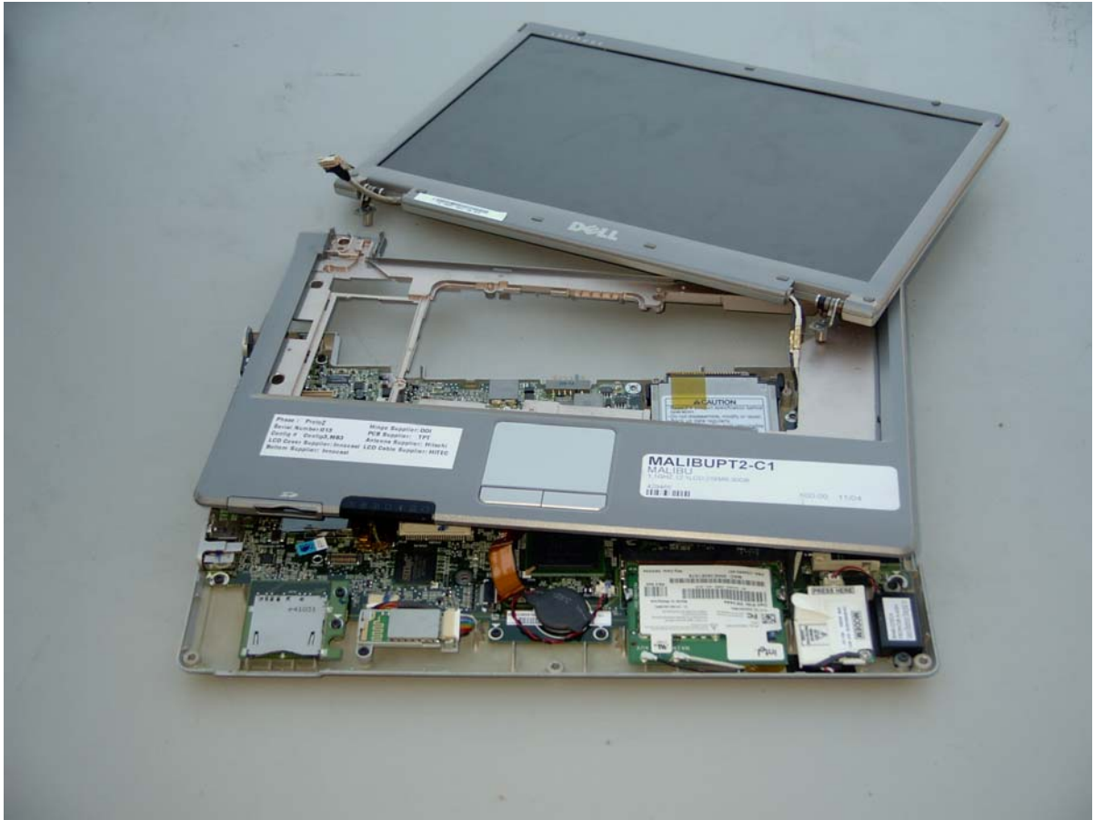
View of the WLAN Transmitter Location Inside the Laptop
