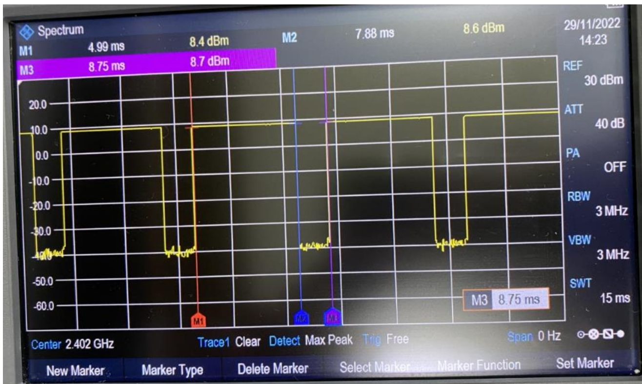
Time-domain plot for Bluetooth transmission signal
