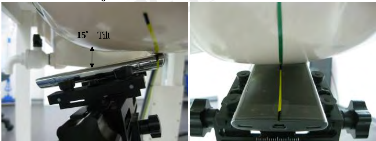
Fig.6 Left Head Section / Ear-Tilt Position(15°)
