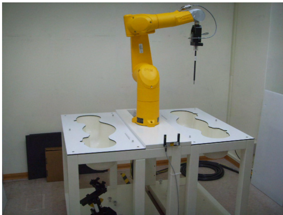
Fig.1 Photograph of the SAR measurement System
