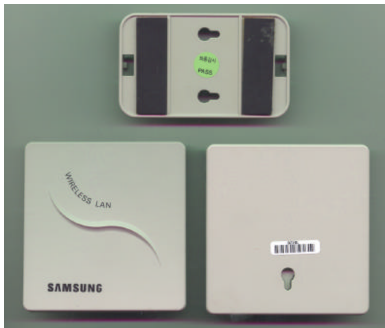
Figure 22: ISA Antenna Outside Bracket & Cover
