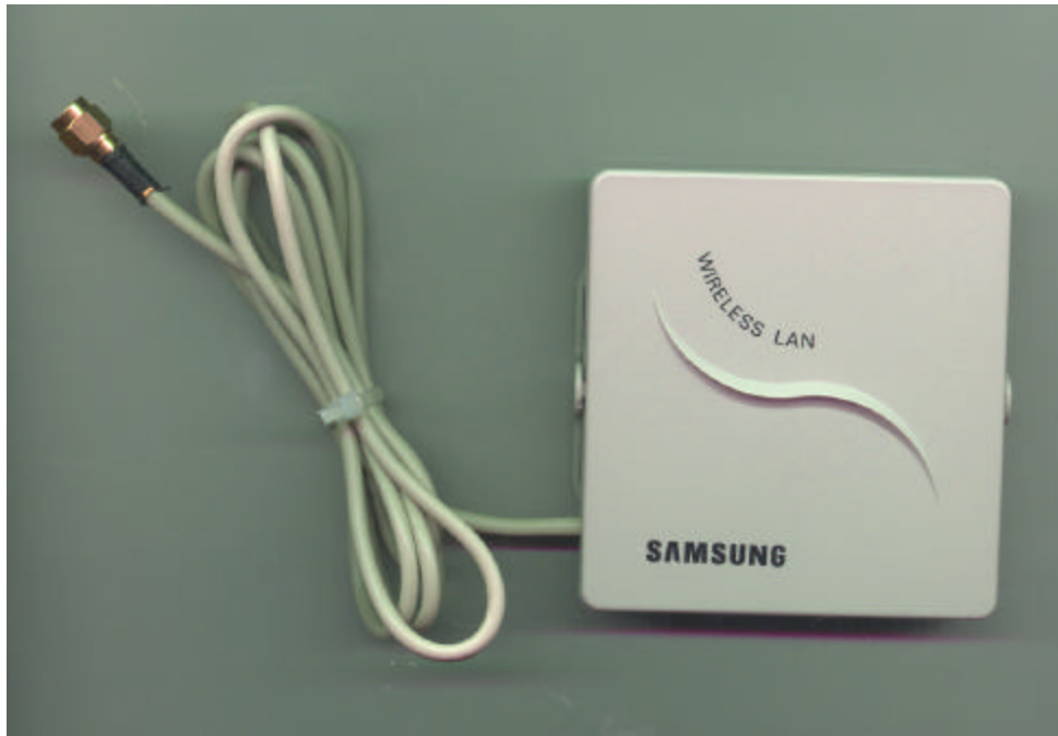
Figure 19: ISA Antenna (Front)
