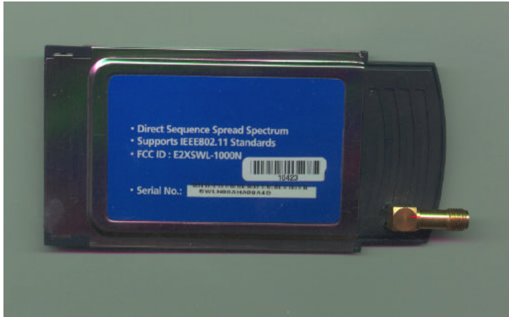
Figure 26: PCM with Stub, Back
