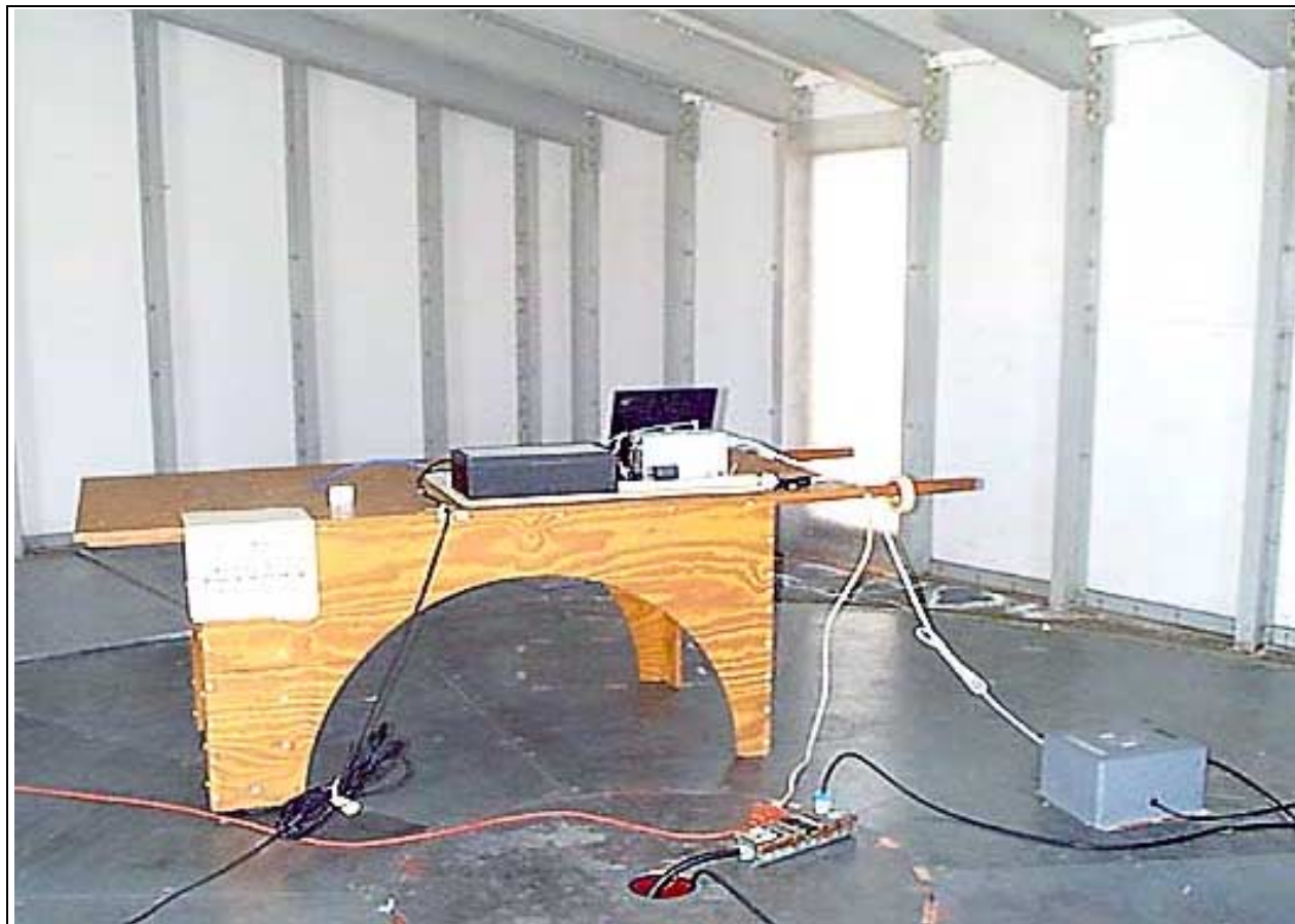
Mains Conducted Emissions - Back View - LRP-PT-ANT06
