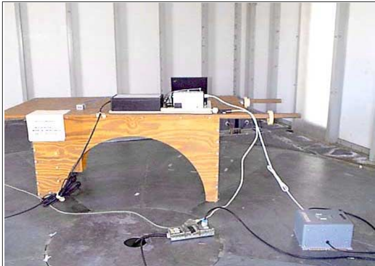
Mains Conducted Emissions - Back View - LRP-PT-ANT03
