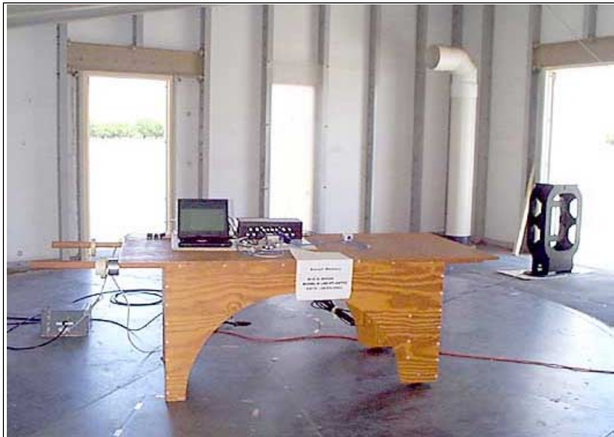
Mains Conducted Emissions - Front View - LRP-PT-ANT03
