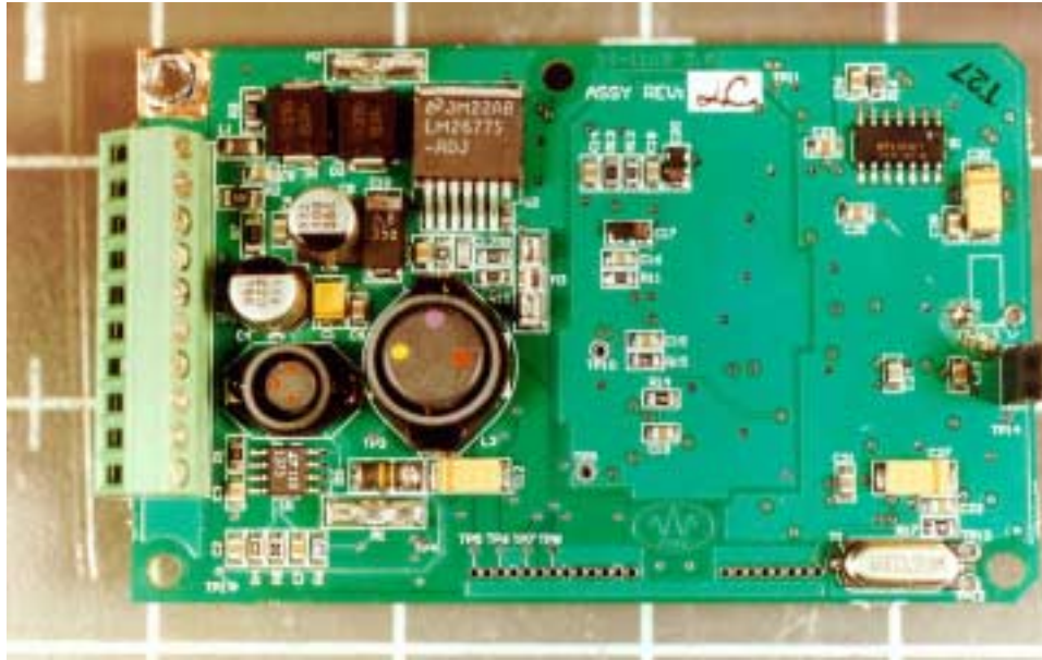
Bop Main PCB without shield over power supply
