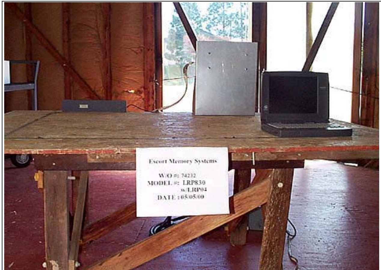
Radiated Emissions - Front View with Antenna 04
