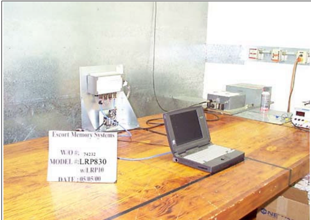
Conducted Emissions - Front View with DC Load
