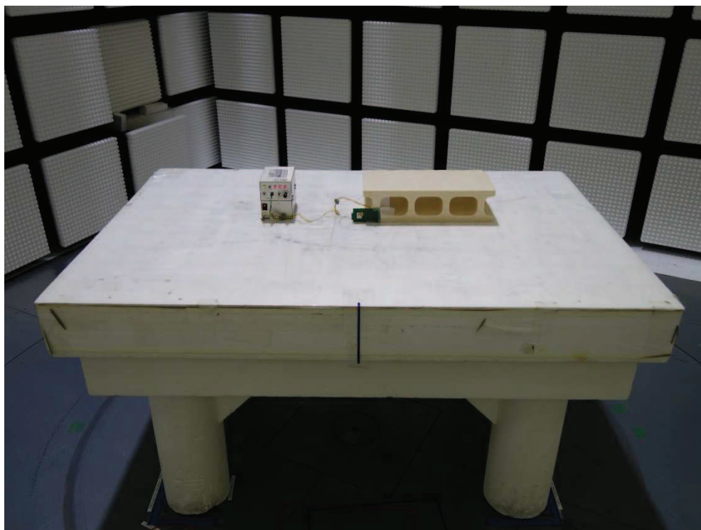
Photograph 7: Set-up for Radiated Emission of Transmitter, Front View, Conf2 (Stand-Alone)
