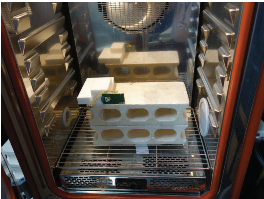
Photograph 2: Set-up for Frequency Stability, inside Temperature Chamber, Conf1 (Stand-Alone)
