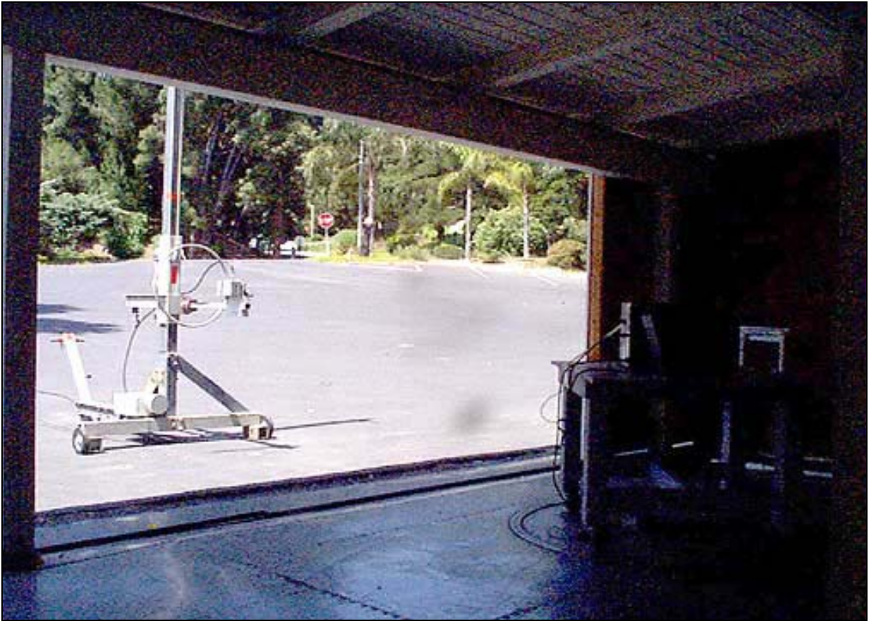
Radiated Emissions - Front View - Loop Antenna
