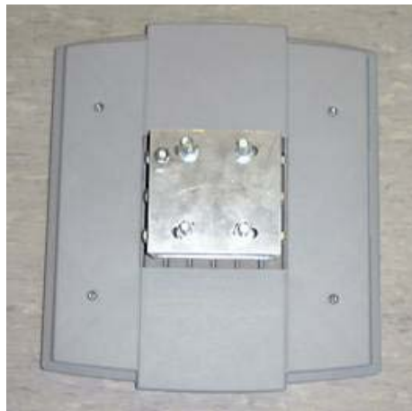
Figure 3-8. MDS 5800 II ODU Rear View
