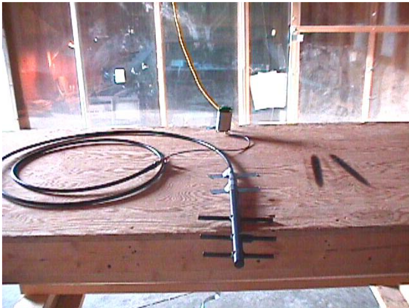
EUT with MDS ClearWave Yagi Directional Antenna
