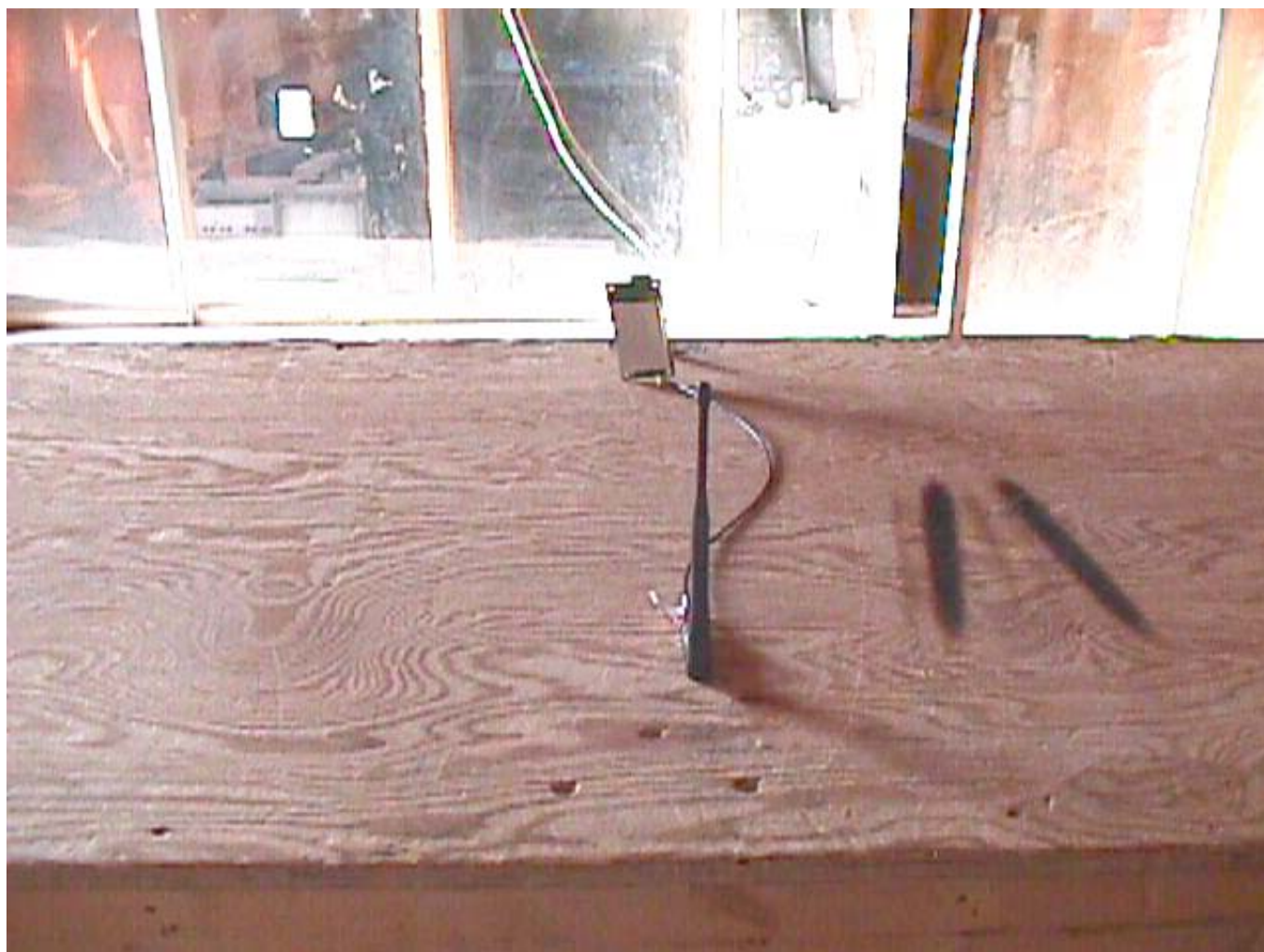
EUT with MDS ClearWave ½ Wave Dipole Antenna
