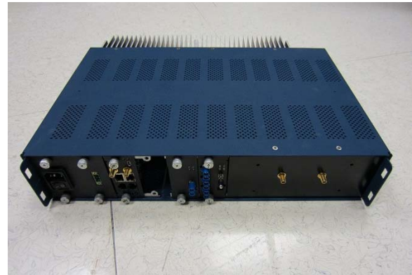
Figure 2: Typical Orbit MPRS Master Station Chassis. The SDM4-1 modules may be installed in any free peripheral slot of this chassis.
