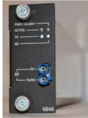
Figure 6-7. SD Radio Module (Part No. 03-6846Axx—SDM9)
