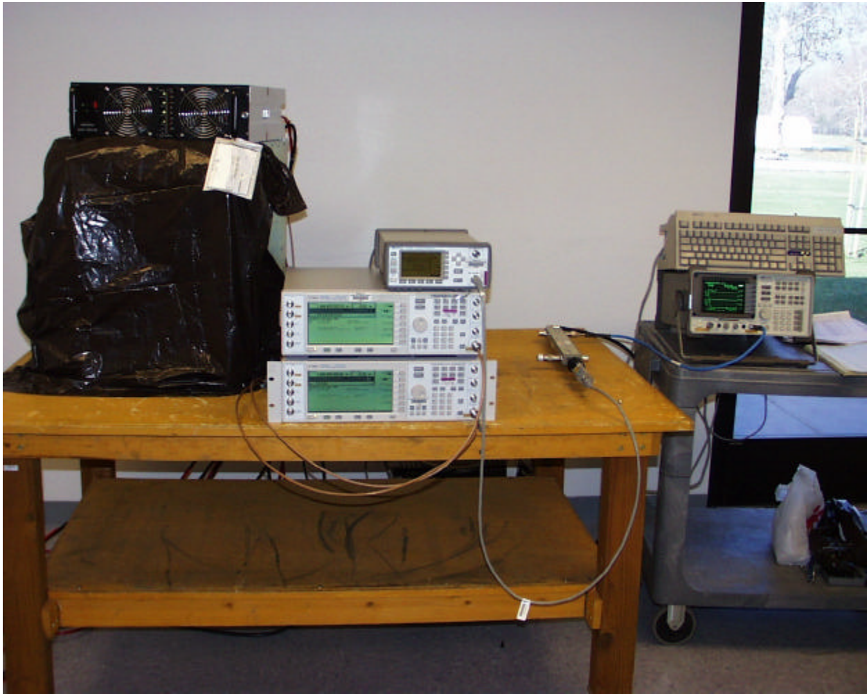
Spurious Emission at Antenna Terminal setup
