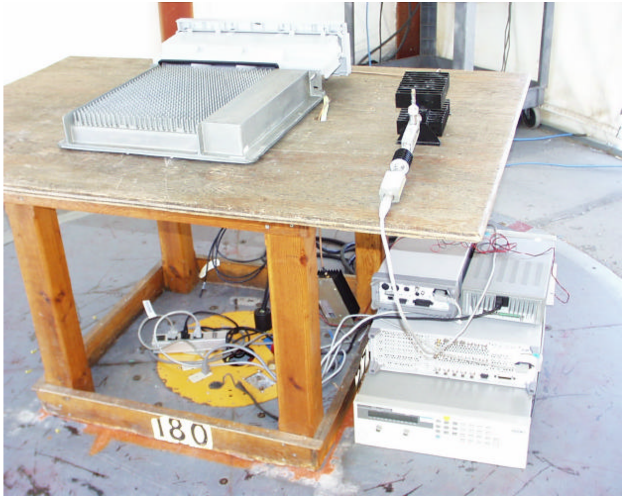
Part15 back view Radiated Emission Setup
