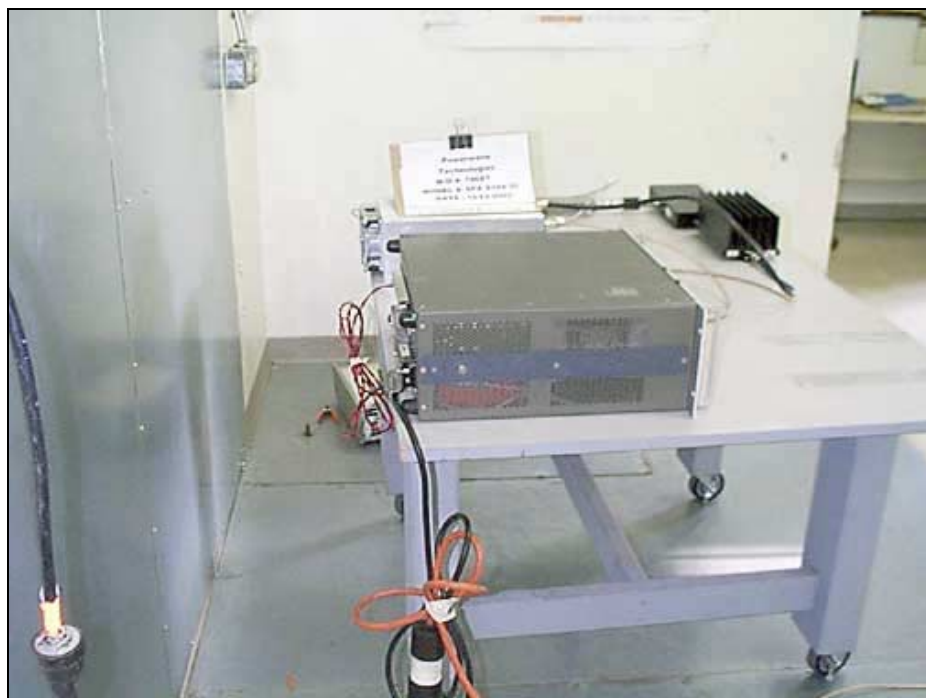
PHOTOGRAPH SHOWING MAINS CONDUCTED EMISSIONS
