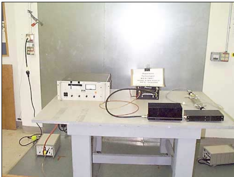
PHOTOGRAPH SHOWING MAINS CONDUCTED EMISSIONS
