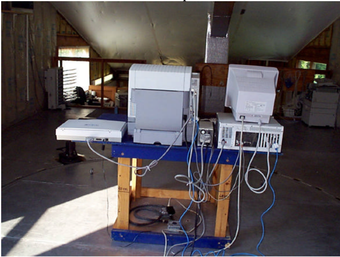
Radiated Test Setup - Rear View
