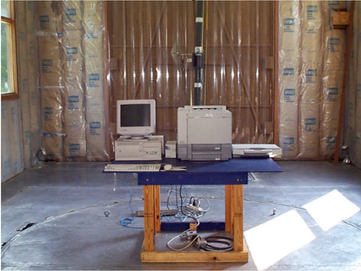
Radiated Test Setup - Front View
