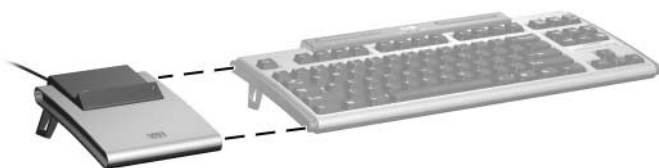
Attaching the Smart Card Adapter to the Modular Keyboard
