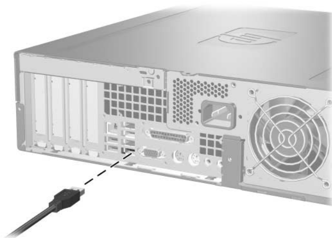
Connecting the USB Cable to the Computer
