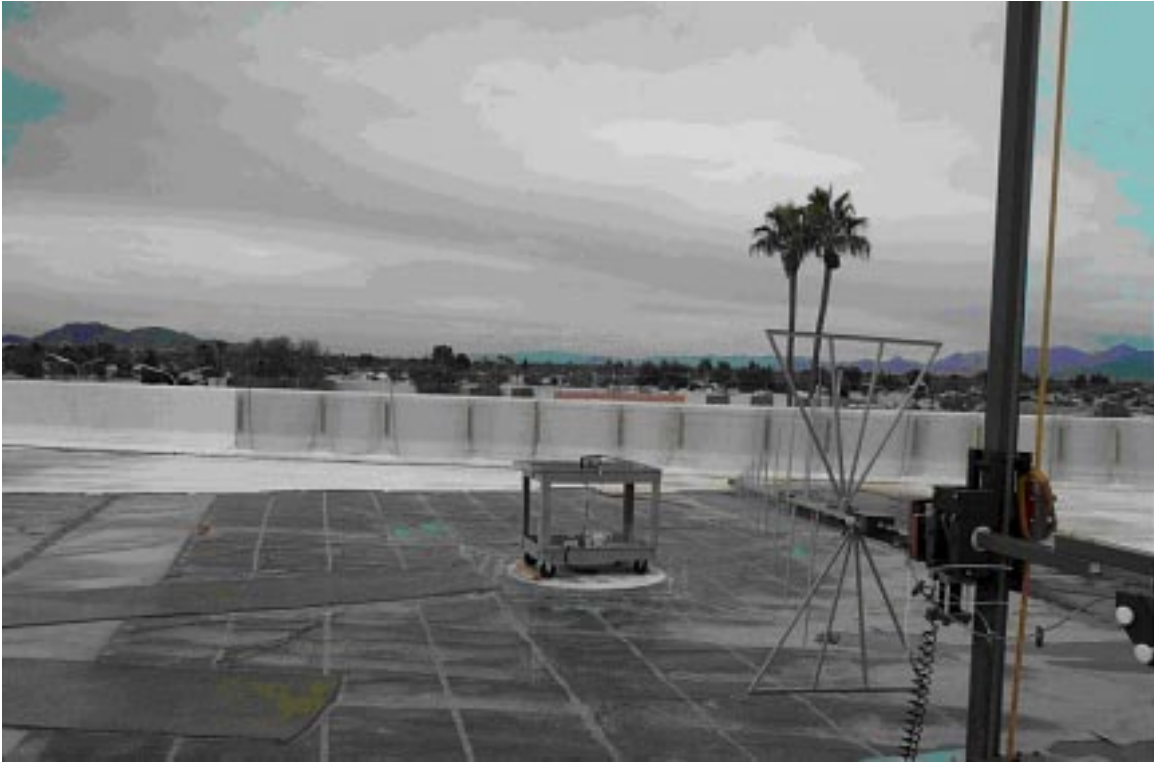
Figure C – 1 Radiated Spurious Emissions Test Setup, OATS
