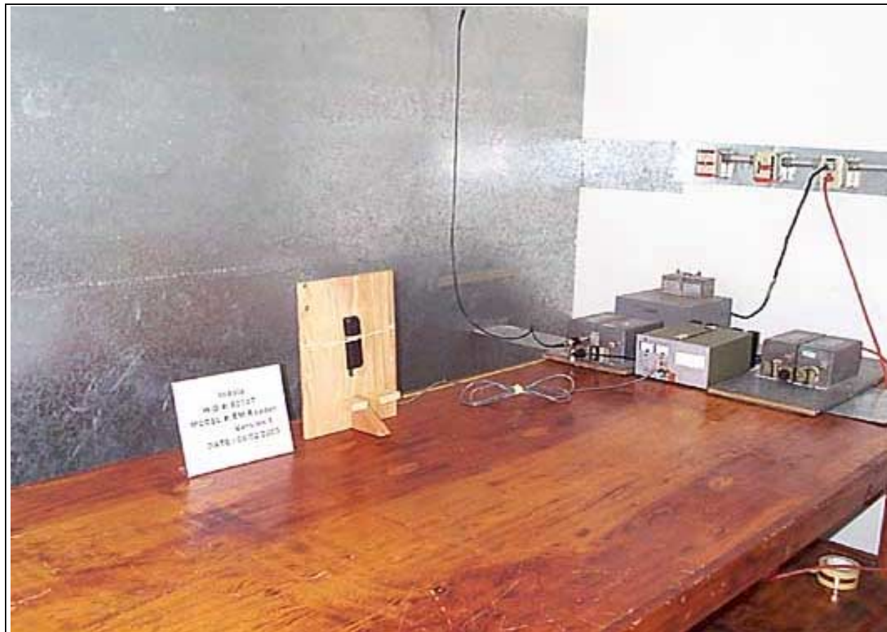
Mains Conducted Emissions - Front View
