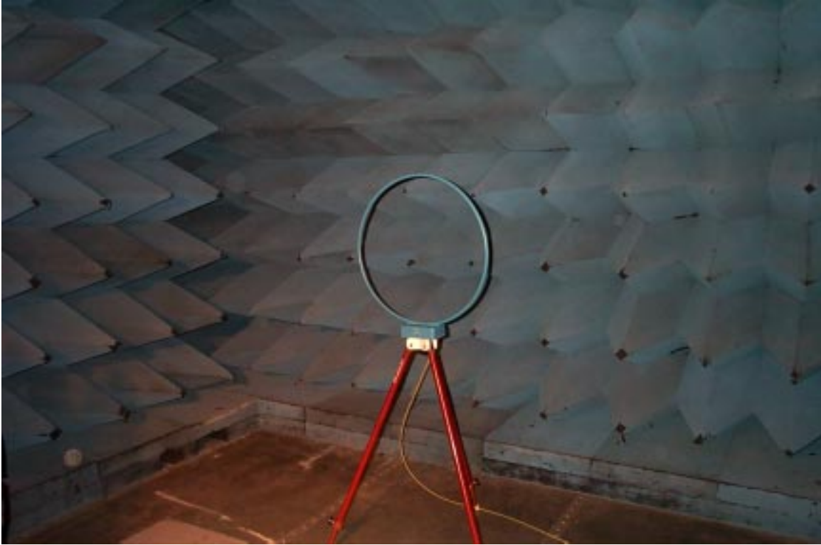
Figure H – 4 Radiated Spurious Emissions Prescan Test Setup, 9kHz - 30 MHz
