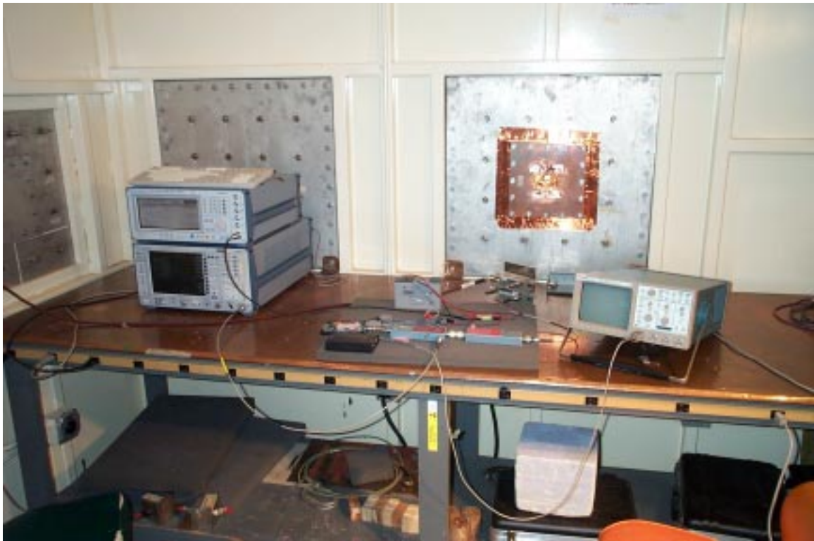
Figure H – 11 Processor Gain Test Setup; Inside Shielded Enclosure
