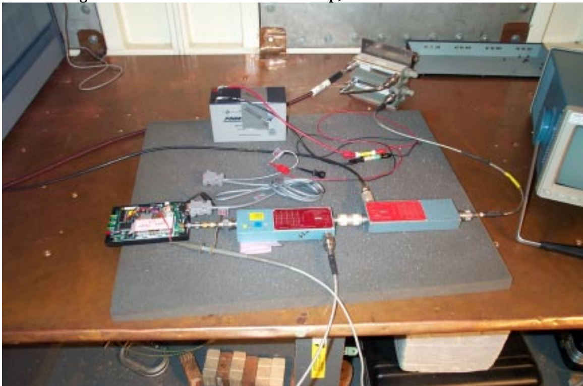
Figure H – 12 Processor Gain Test Setup; Inside Shielded Enclosure (Closeup)
