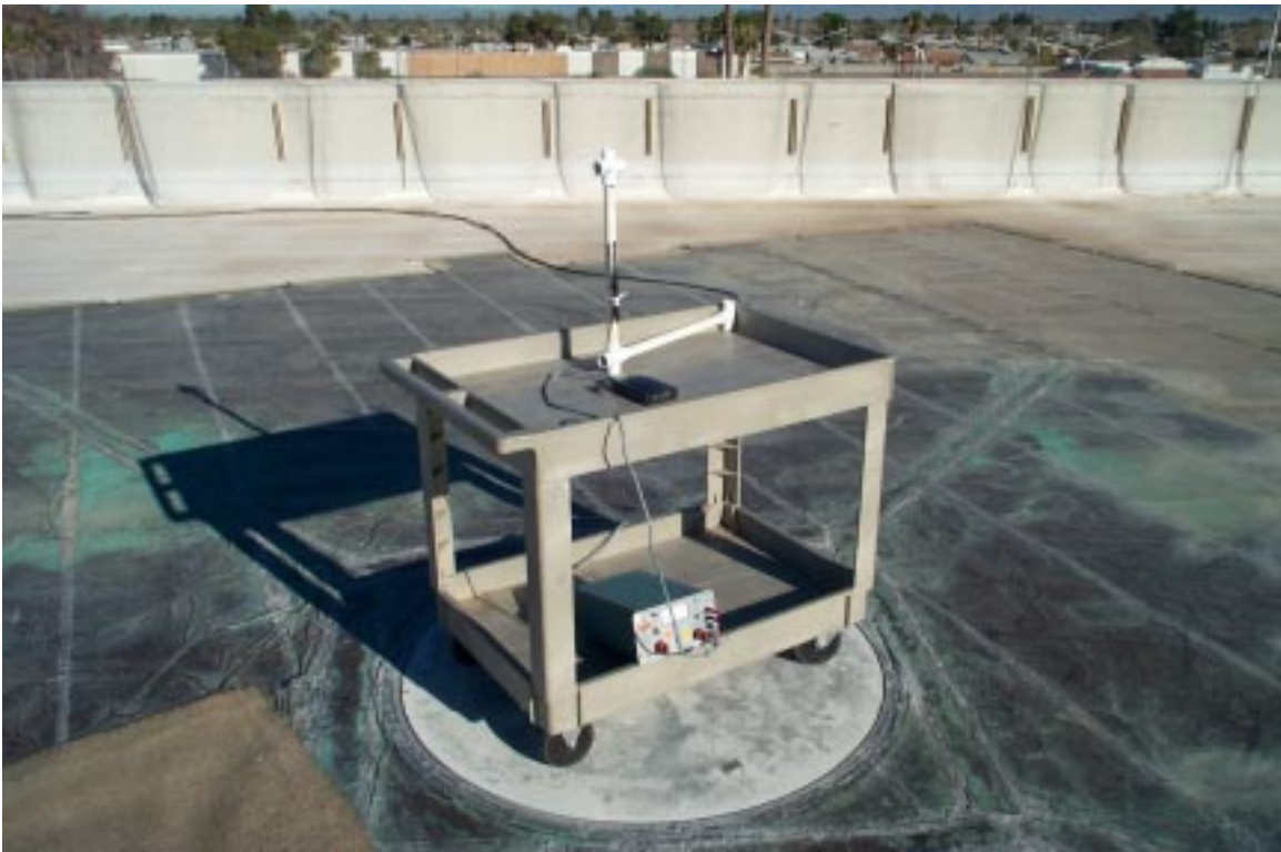
Figure H – 9 Mobile Station; Radiated Spurious Emissions Test Setup, OATS Setup
