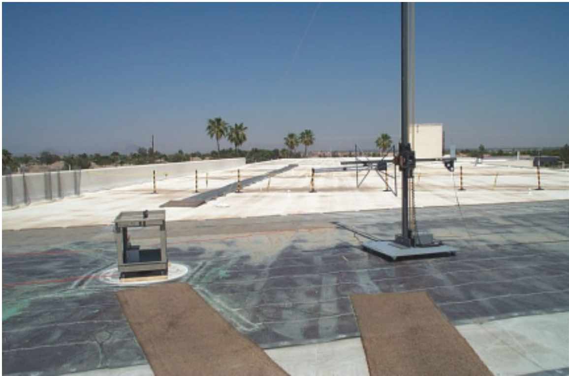
Figure C – 3 Radiated Spurious Emissions Test Setup, OATS
