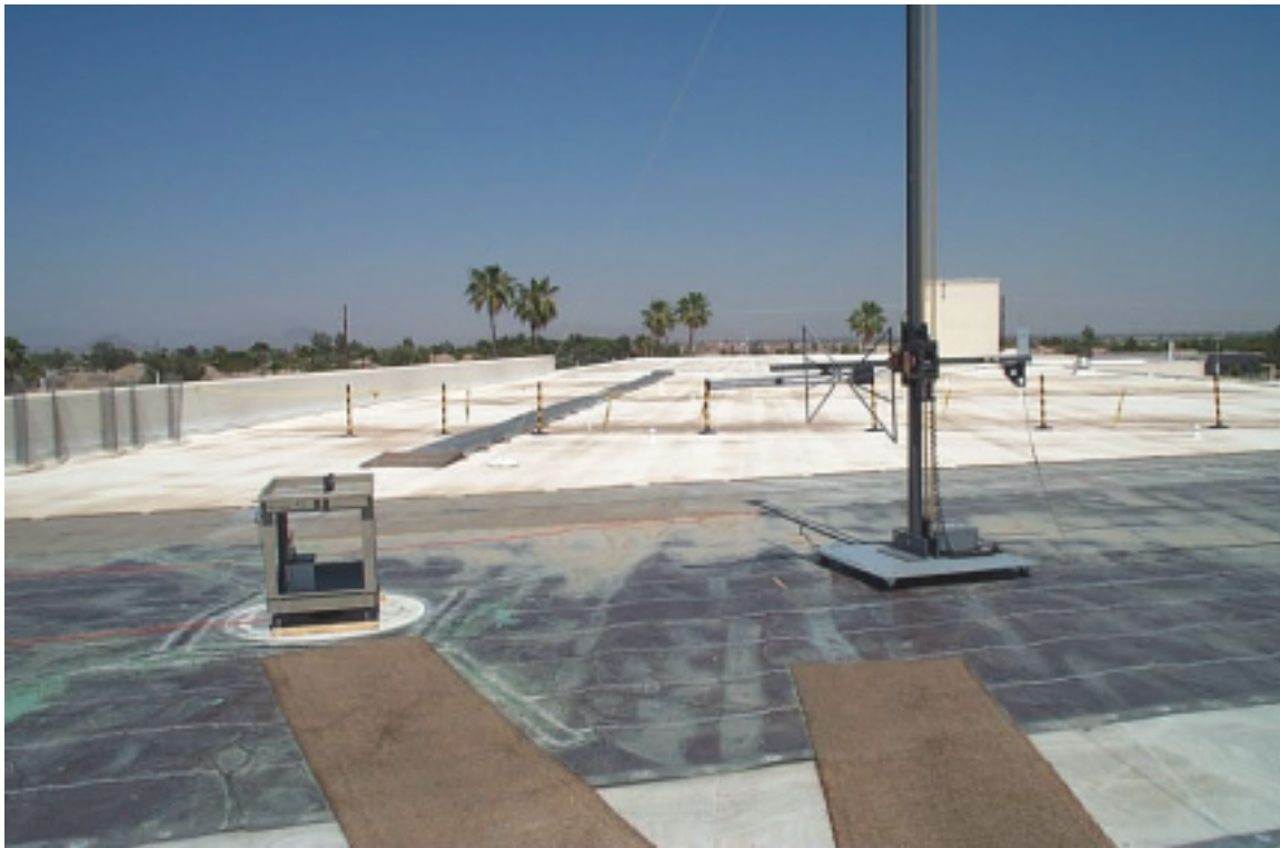
Figure C – 3 Radiated Spurious Emissions Test Setup, OATS
