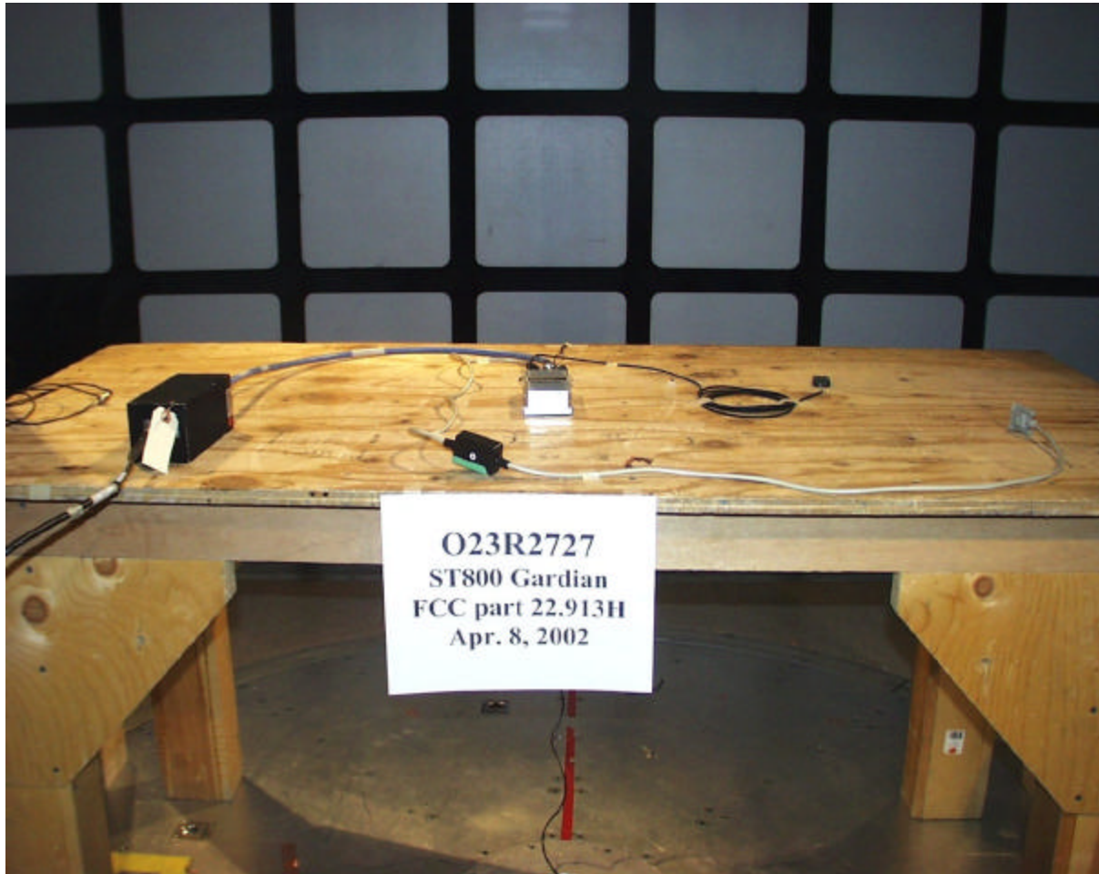
FCC Part 22.913 ERP measurement setup
