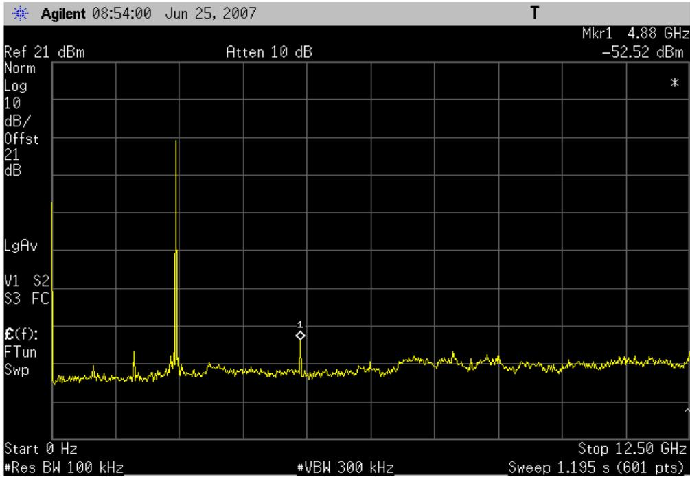
Mid Channel, QPSK (Middle Data Rate 2DH5), 12 - 25 GHz
