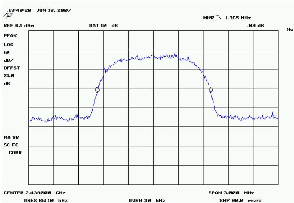
QPSK (Middle Data Rate 2DH5), High Channel
