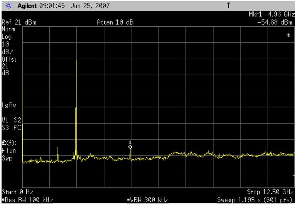
High Channel, QPSK (Middle Data Rate 2DH5), 12 - 25 GHz
