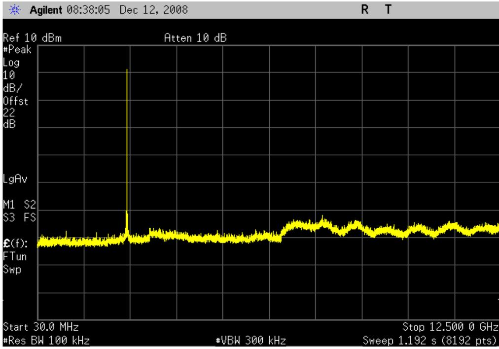
8DPSK, 3DH5, Mid Channel, 12.4GHz-25GHz
