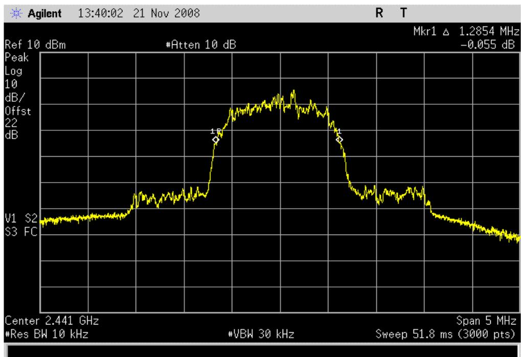
8DPSK, 3DH5, High Channel, 2480 MHz
