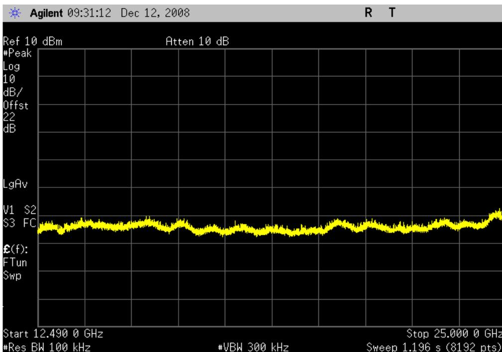
8DPSK, 3DH5, Mid Channel, 30MHz - 12.5GHz
