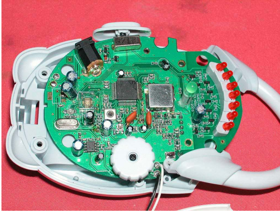
Main PCB comp side
