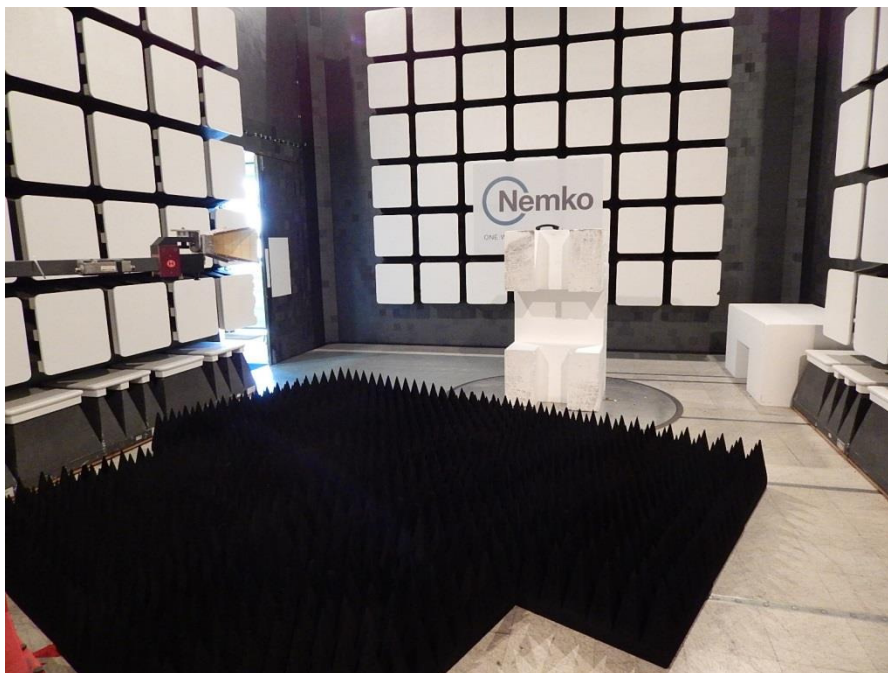
Figure 8.5-71: Radiated spurious (out-of-band) emissions setup photo – above 1 GHz
