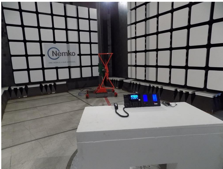
Figure 8.6-70: Radiated spurious (out-of-band) emissions setup photo – 30 to 1000 MHz
