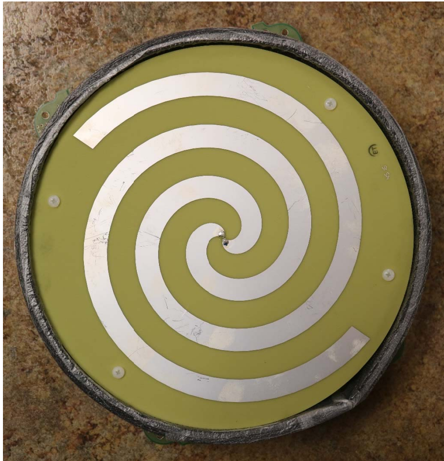
4-00203 ORION 900 ANTENNA / RF BOARD ASSEM– Side B:
