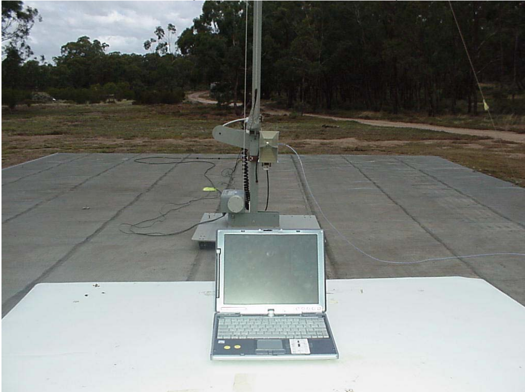
Radiated Emissions Test Setup (3 metre distance - Harmonics)
