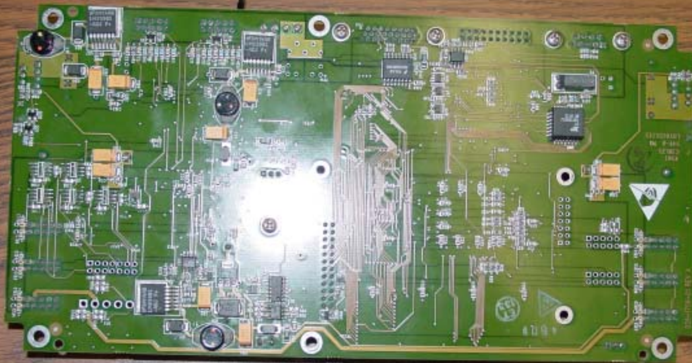
087-1706-01 Alarm Control Unit (Back)
