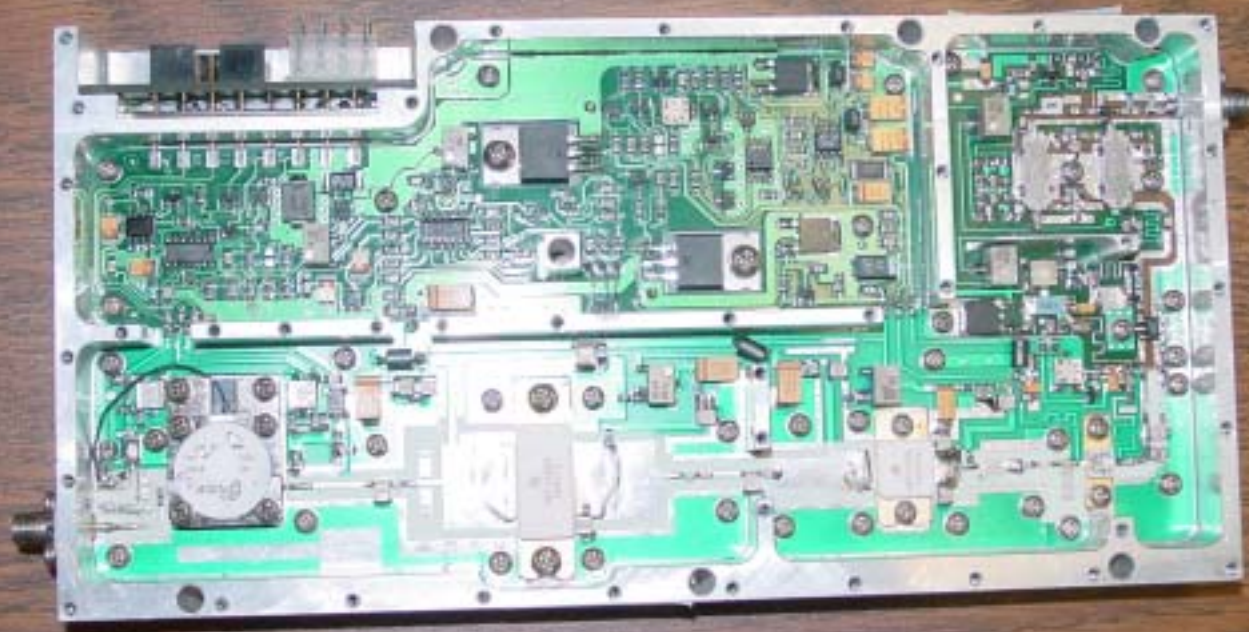
149-1011-01 Forward Power Amp (Front) RF Module
