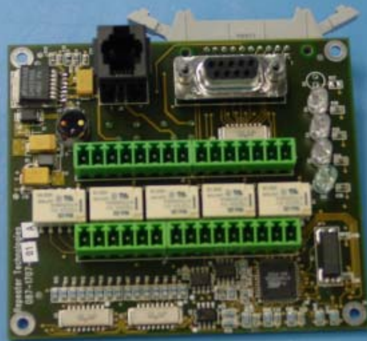
087-1707-01 Line Entry Module (Front)
