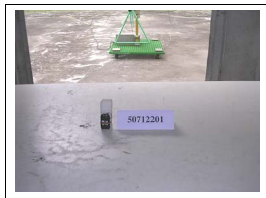
Radiated Open Site Test Set-up
