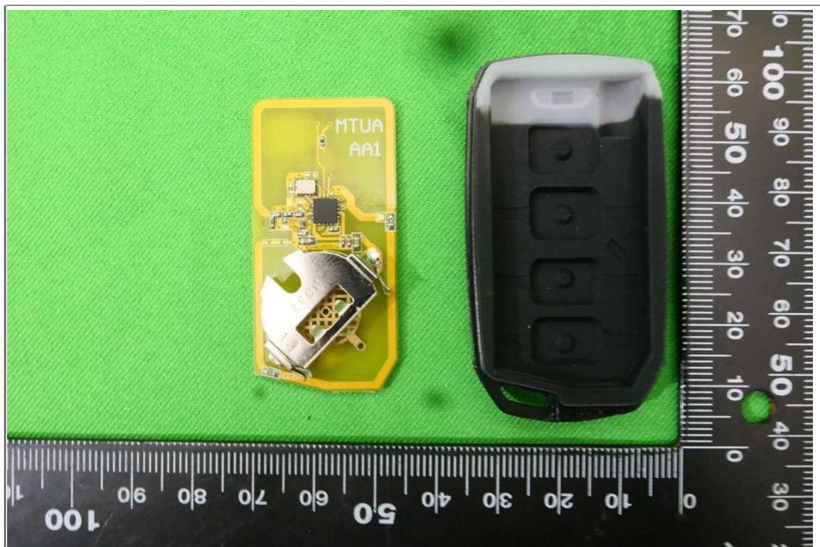
Inner View of EUT-2
