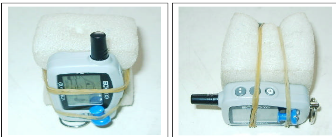
Radiated Open Site Test Set-up (Transmitter Mode)
