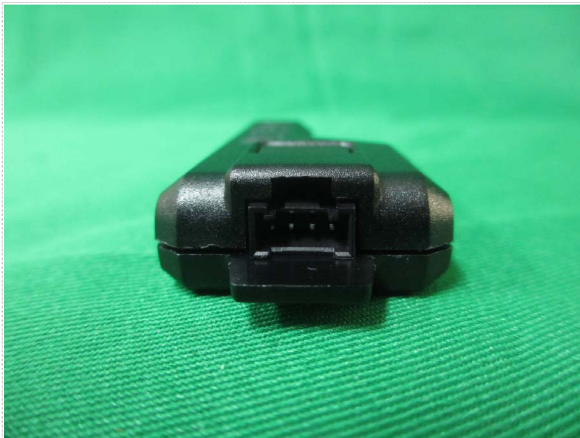
View of Power port
