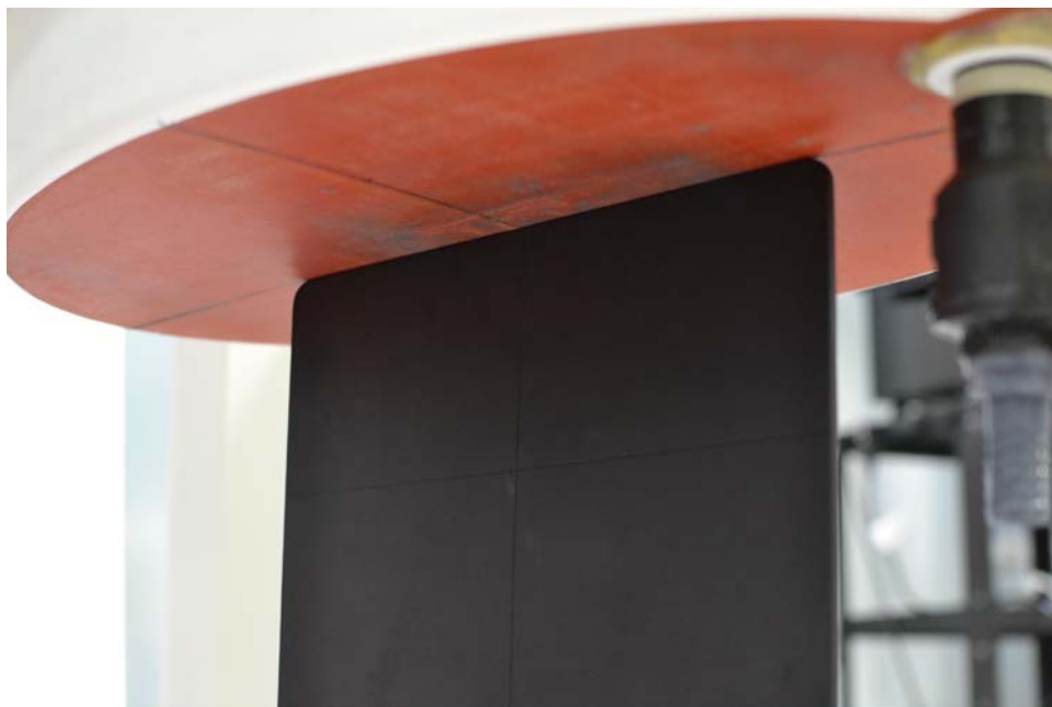
SAR Test Setup Photo 1 – Front Edge at 0 mm
