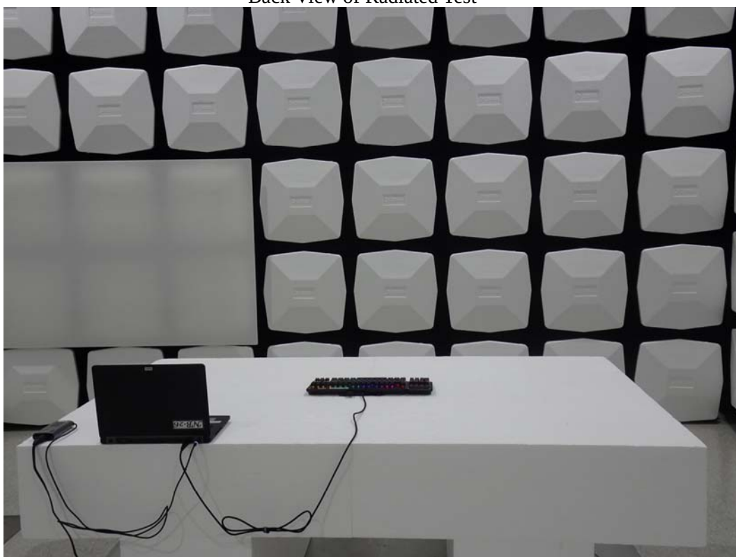
Back View of Radiated Test
