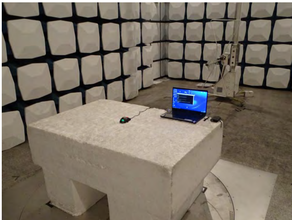
Back View of Radiated Test
