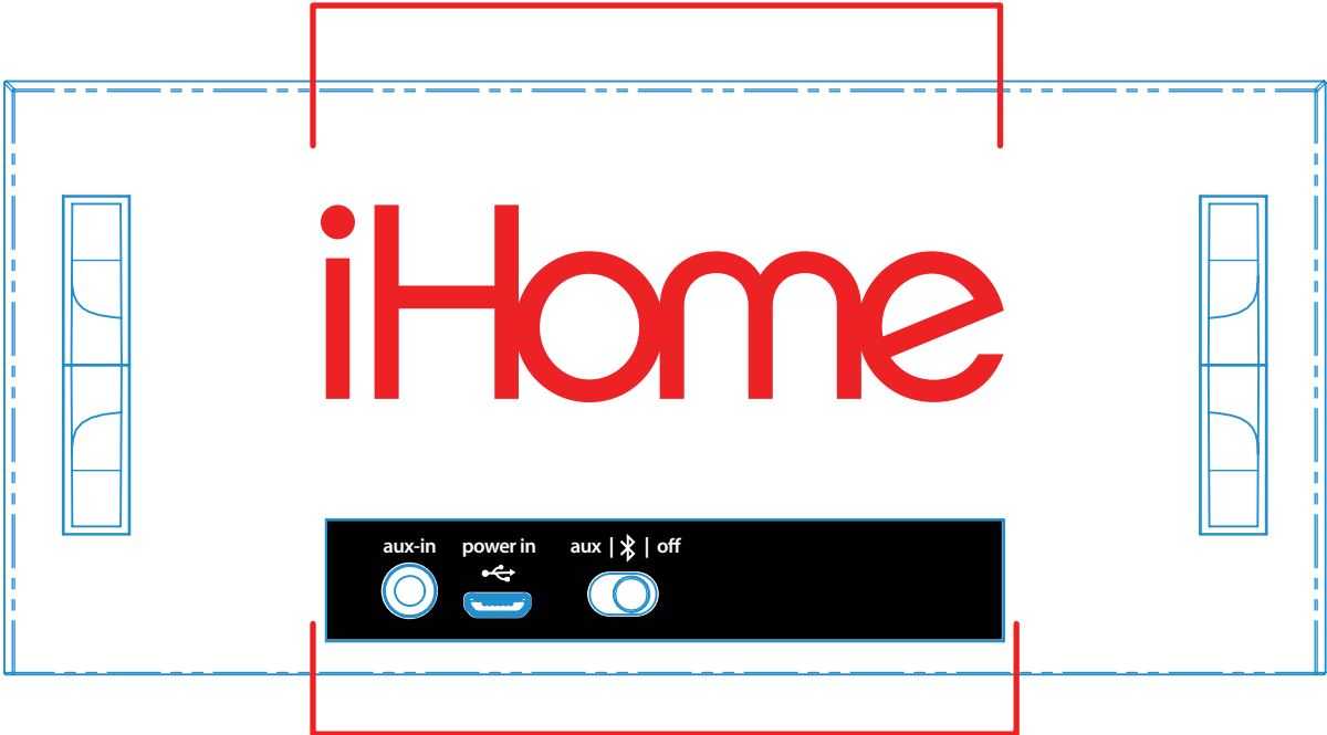
Rear Panel PVC Cut Sheet: Same as model plate material, matte finish. see rendering for color.
