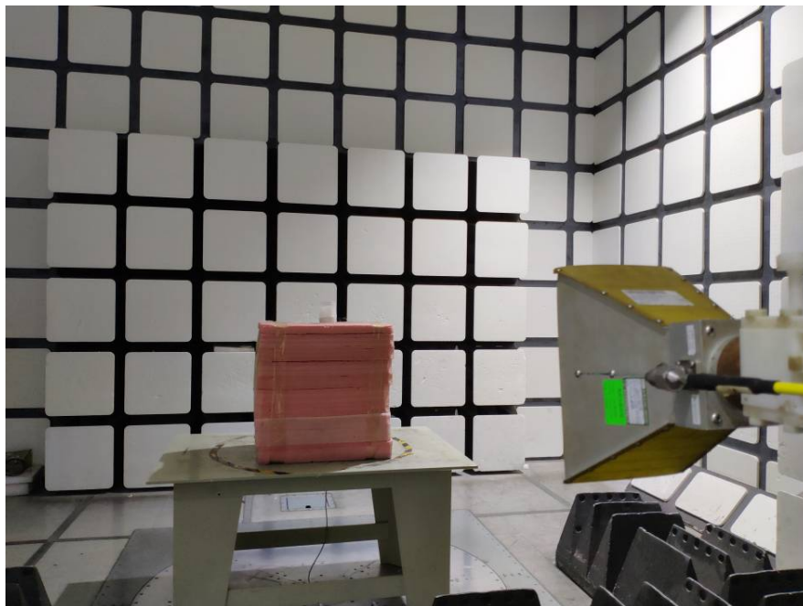
Radiated Emissions View (Above 1 GHz)
