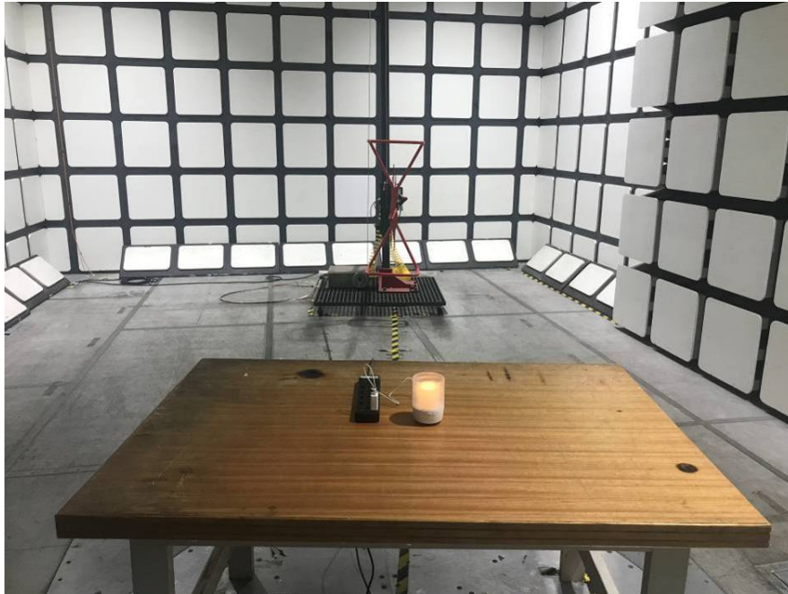
Radiated Emissions View (Below 1 GHz)
