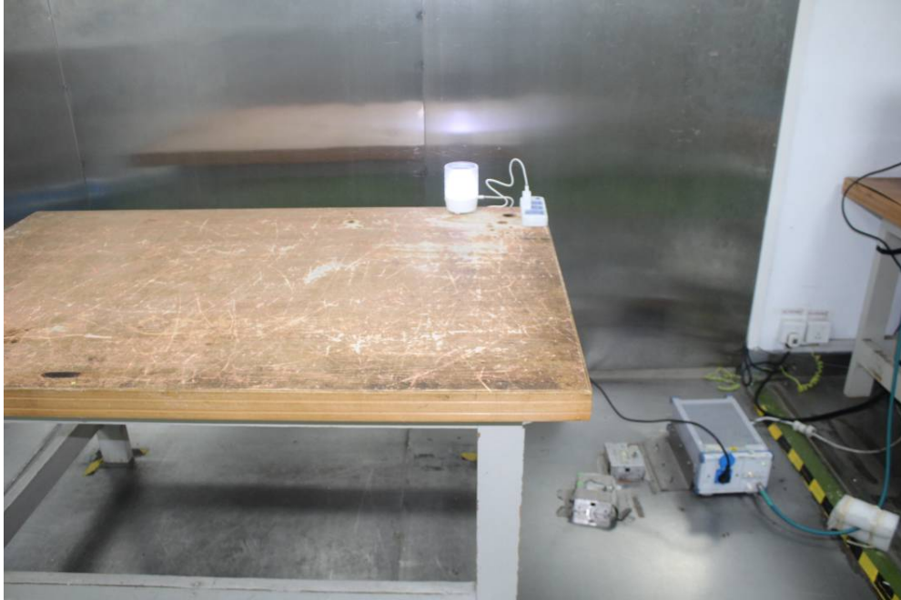
Conducted Emissions - Front View
