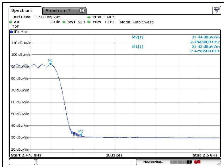
Higher edge (Bluetooth 3.0, Average measurement, hopping mode)
