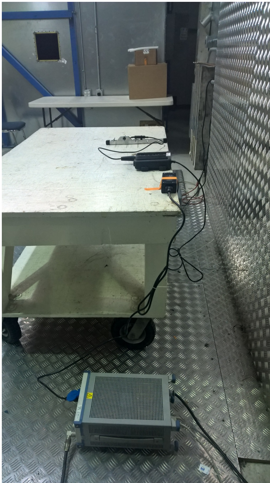
Figure 8.2-3: Conducted disturbance at mains port setup photo
