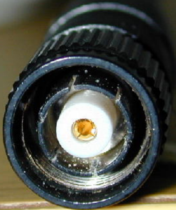
"Ducky" Antenna Connector - Reverse TNC
