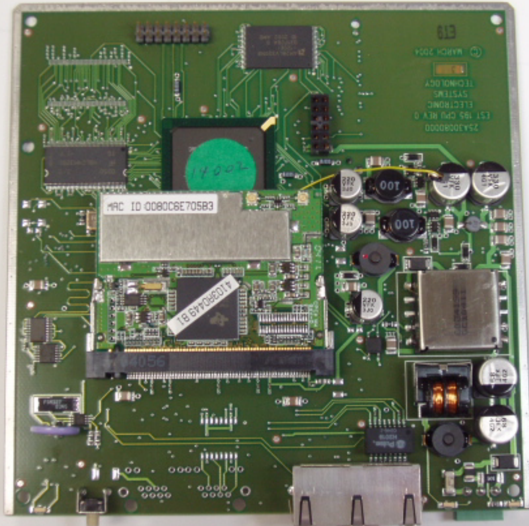
CPU Board with Radio Board Installed
